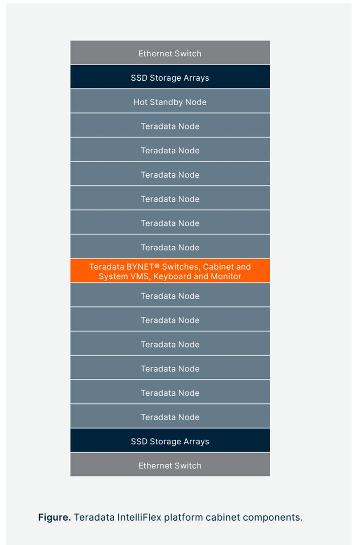
Figure. Teradata IntelliFlex platform cabinet components.
