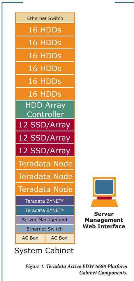
Figure 1. Teradata Active EDW 6680 Platform Cabinet Components.
